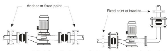
Rubber bellows will exert a pressure thrust in service and must be anchored to protect adjacent pipework and equipment. Rubber bellows will extend under pressure and must be anchored to prevent this happening.
