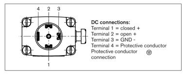
The connection terminals in the cable plug are identified with the numbers 1 to 3 according to the terminals on the valve.
