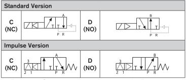
→ Type 0344: Connect vacuum pump to connection R.
