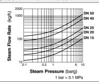
The chart to the left is used to determine the steam flow rate through the SF1 separator-filter. It is based on a steam velocity in the piping of 30 m/sec. For other velocities, calculate the flow rate as follows:
