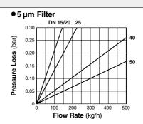
These pressure loss charts are based on a steam pressure of 1 barg. For other pressures, multiply the steam flow rate by the correction factor given in the table right. Use the result on the pressure loss chart.
